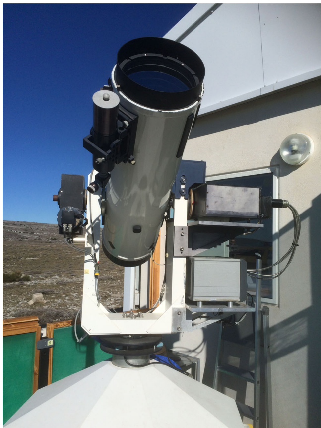
Figure 1. MISOLFA instrument with its entrance window, the alt-azimuthal mount and its focal box on a Nasmyth focus (on the top). In the bottom, we can see the pupil-plane amplification device. The two boxes are connected with optical fibres.
