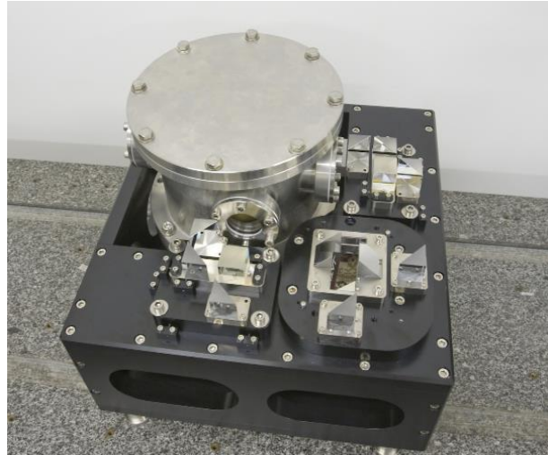
Figure 2. View of the DSI instrument during integration phase. The Mach-Zehnder is inside the vacuum chamber on the left. The two output beams are splitted by polarizer cubes and folded onto the detector, that will take place above the mirrors, on the right.
